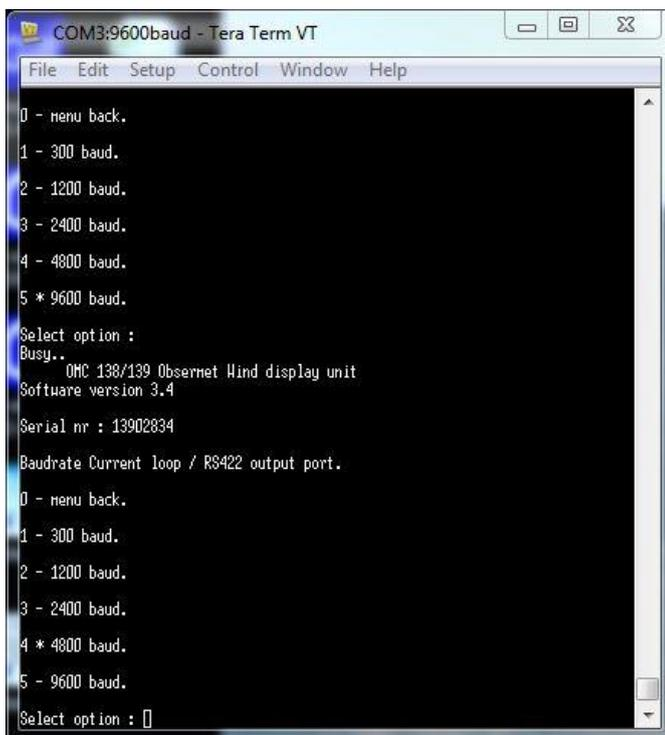
Once done, press '0' 3 times to return to the main menu. The settings can then be checked by selecting option 5 'show all settings' to ensure that they have been successfully changed:
