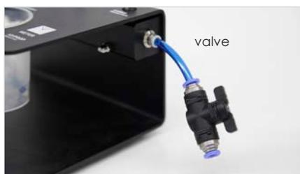
Timer starts the pump automatically and works in the rhythm set. The water in the tensio shafts is degassed after minimum 24 hours running time.
