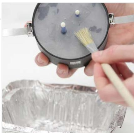
Clean also sample ring and silicone gasket above the bowl to avoid losses.
