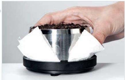
Fill 2 cm (1 in) of degassed water into a tray. Put the soil sample into the tray – tilt it so that air under the soil can escape.
