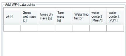
The gravimetric water contents are calculated automatically, converted into volumetric water contents, and added to the graphics. When fitting the hydraulic properties these data have the same weighing factor as the HYPROP data. Power user may change this factor.
