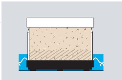
Raise the water level up to 5 mm below the sample rim (recommended times see below). Do not pour water on the sample – you may trap air. Use the time table below as a reference to determine how long samples take to saturate.
