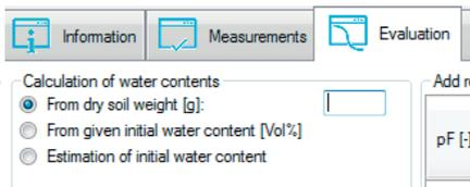
Enter the WP4 value of pF, gross wet mass (wet soil + cup), gross dry mass (dry soil + cup) and tare mass (cup only) in the register "Evaluation" and the table "Add WP4 data points". This can be done by cut and paste from a spreadsheet.
