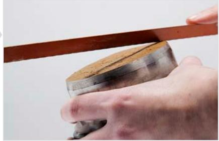
Put a plastic cap upside down on the sample ring – on the side where the ring has the cutting edge. The cap works as a support. This makes sure that no soil gets lost even when loose sand is in the sample ring.
