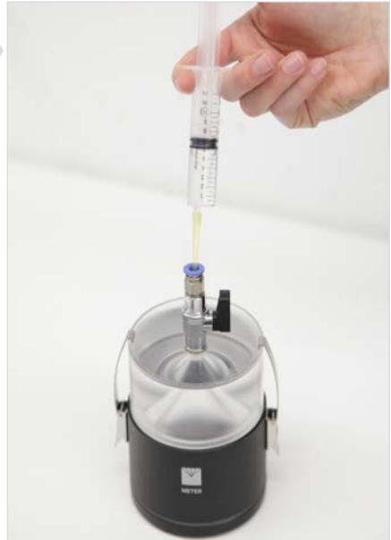
Fill vacuum syringe with 15 to 20 ml deionized water. Degas water in the syringe as explained on the previous pages.
