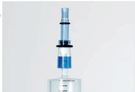
Fill vacuum syringe with 5 ml deionized water. Turn syringe upside down and remove residual air.
