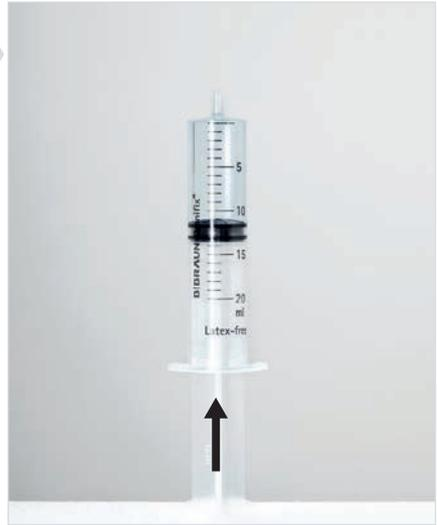
Push tube piece onto the tip of the syringe. Push plunger of the syringe until a meniscus builds up on the tube piece.
