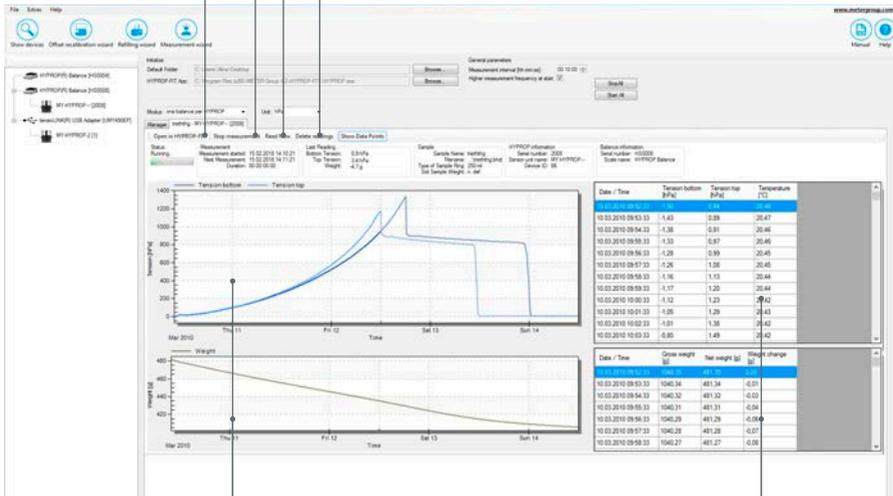
Display of the soil sample's tensions and weights over time (graphical)
