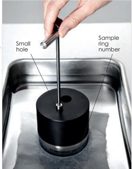
Fill drill holes with water to make sure air will not be pressed into the soil sample during assembly.
