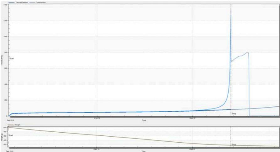
Material: packed quartz sand particle size: 0.1 bis 0.3 mm, soil type: sandy sand (S: 100%, U: 0%, T: 0%), site: Bodenphysikalisches Labor, TU Braunschweig, evaporation: 1.4 mm/d, temperature: 22°C
