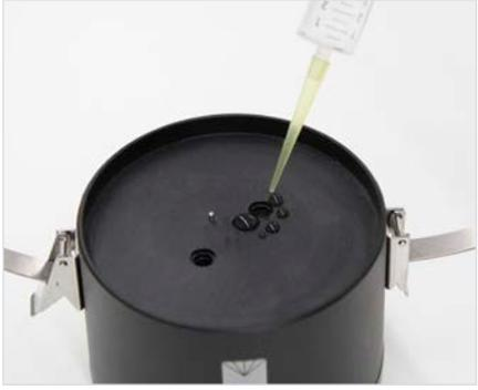
Set up refilling attachment and fix it. Fill attachment with droplet syringe – ideally bubble free.
