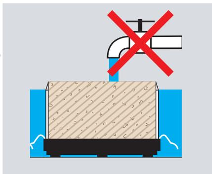
Let soil sample capillary saturate until the surface is shining.
