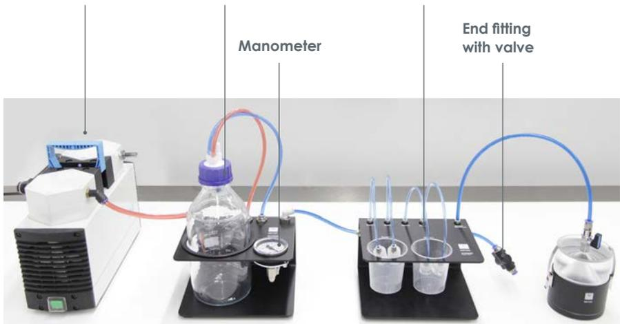
Put the vacuum pump on the ground (lower temperature) to gain better vacuum values.
