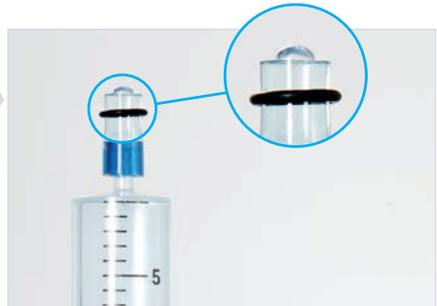
Connect the two syringes and the tensio shaft.
