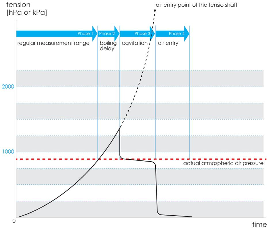
The four phases using one tensio shaft as example
