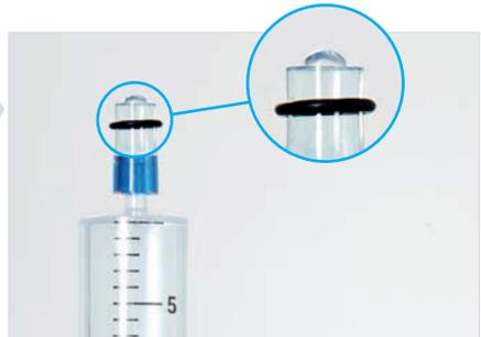
Push the ceramic of the first tensio shaft into the tube piece.
