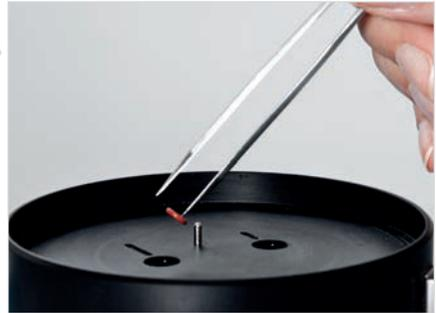
Take the spare O-ring from the service pack. Do **not** pierce it. Put O-ring into the hole and let it "snap" into the groove on the bottom. If the O-ring does not snap in itself screw in the tensio shaft cautiously.
