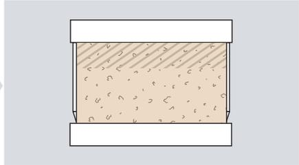
Turn soil sample upside down and put it on a table. Remove cap on top, place nonwoven cloth on the soil and put the filling bowl on the sample ring.
