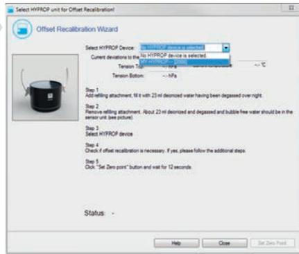
Check if the device recommends a recalibration.
