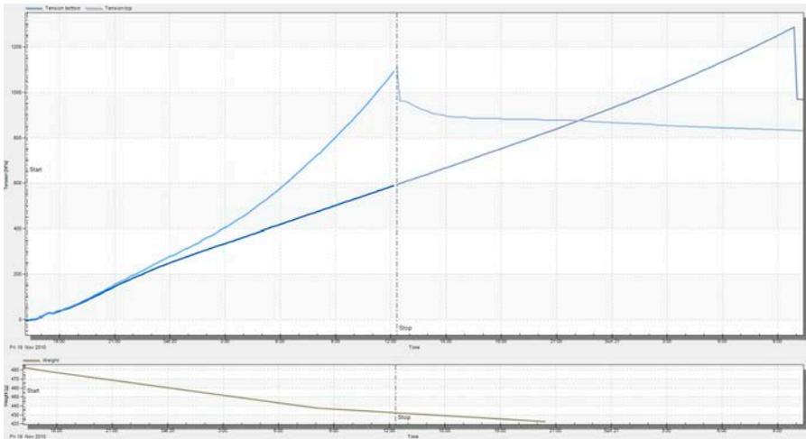
Site: Groß-Gleidingen near Braunschweig; soil type: clayey silt (S: 1%, U: 82%, T:17%); measurements: Praktikum Bodenphysik at TU Braunschweig, 2010. Evaporation: 14 mm/d using a fan. Temperature: 20°C
