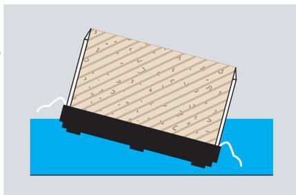
Put a plastic cap upside down on the sample ring. Do not fix it so that air can ventilate. The cap protects the soil from sun radiation and evaporation.
