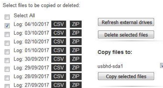
When connecting a USB drive to MetStream after power up then open the Measurement Log screen and click on 'Refresh external drives'.
