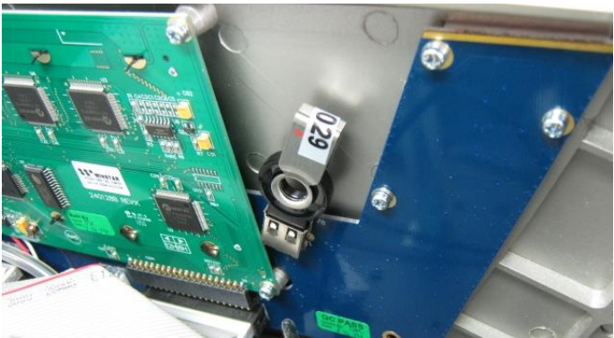
Figure 8 – Installation of USB Memory Key
