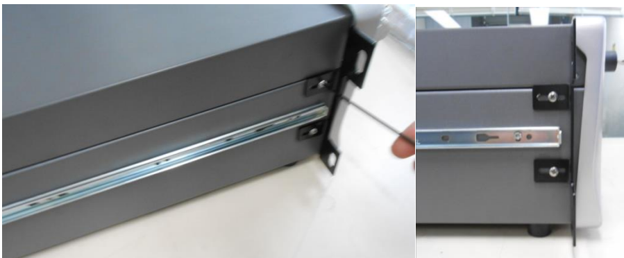
Figure 75 – Rack Mount Ears Fitted to Instrument
