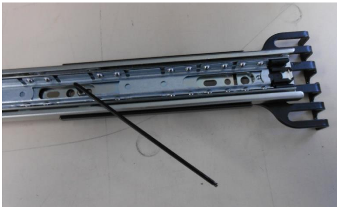
Figure 76 – Attach Rack Mount Adaptors to Outer Slides
