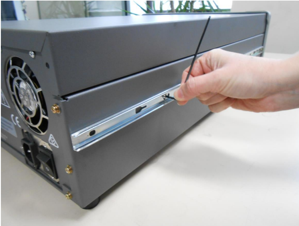
Figure 74 – Assemble Inner Slide on Chassis
