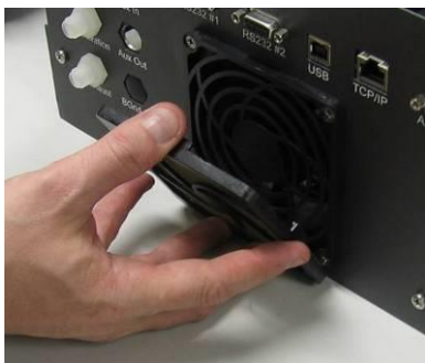
Figure 55 – Removing the Fan Filter
