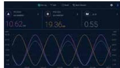
The Centauri's dual channel capabilities enable the user to simply plug in any of Ophir's thermal, pyroelectric or photodiode sensors and measure the two channels independently, or a comparison between the two channels.
