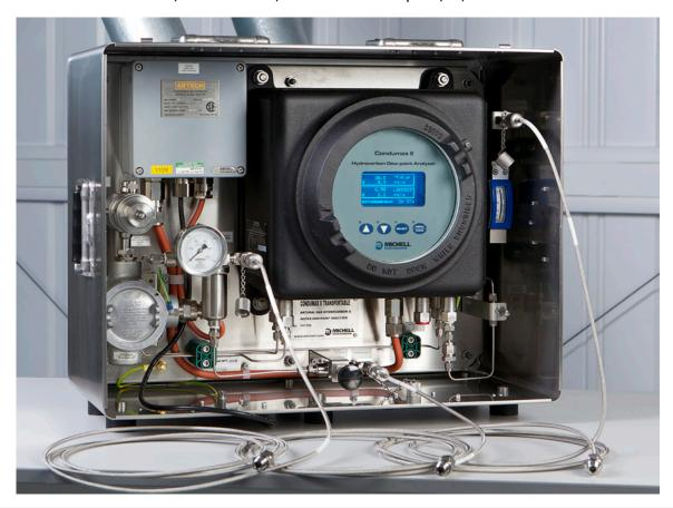
A complete transportable natural gas dew-point analysis system for field spot-check measurements. Periodic online operation when located in a temperature maintained analyzer house. Measurements and functionality are instantly accessible through integrated alphanumeric display and touch-glass HMI interface including log of dew-point readings for operator review.
