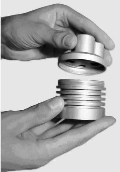
9. Fasten the salt chamber on the holder in the base plate and close the measurement holes with rubber plugs.
