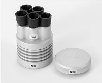
11. Allow approximately 24 hours for stabilization before use so that the salt solution reaches the equilibrium humidity.
