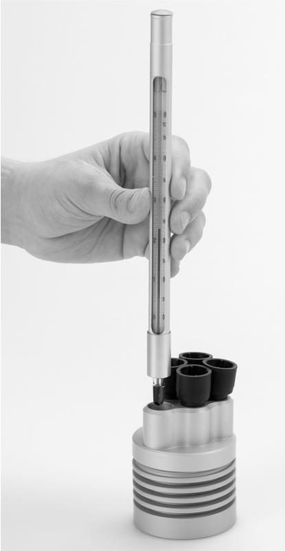
Figure 4 Inserting thermometer
