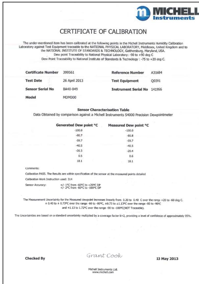
Figure 32 Typical 7-point Calibration Certificate
