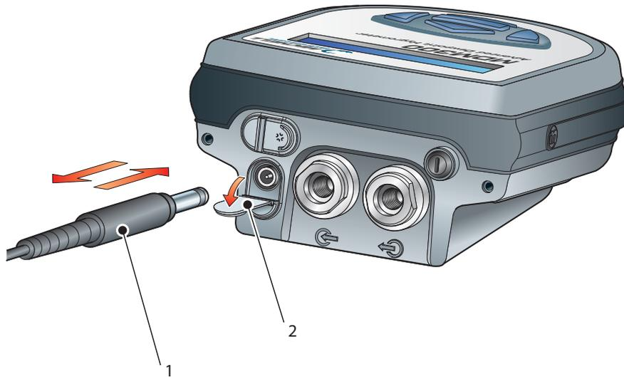
**Figure 14** *Battery Charger Connection*
