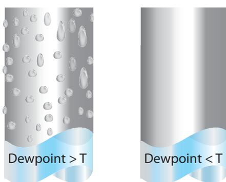
Maintaining the temperature of the sample system tubing above the dew point of the sample is vital to prevent condensation. Any condensation invalidates the sampling process as it changes the water vapor content of the gas being measured. Condensed liquid can alter the humidity elsewhere by dripping or running to other locations where it may re-evaporate.
