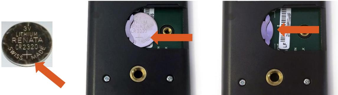
The positive side (designated by a "+" sign) should be facing out from the meter circuit board.
