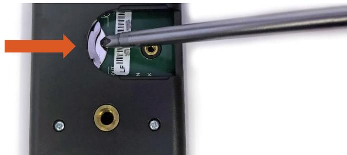
If the battery is difficult to move, turn the meter on its side so that the opening for the battery is facing downward and tap the meter downward against an open palm to dislodge the battery enough so that it can be removed with your thumb to slide the battery out of the battery holder.
