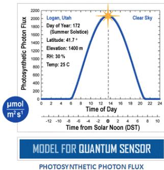
Homepage of the Clear Sky Calculator. Two calculators are available: One for pyranometers (total shortwave radiation) and one for quantum sensors (photosynthetic photon flux).
