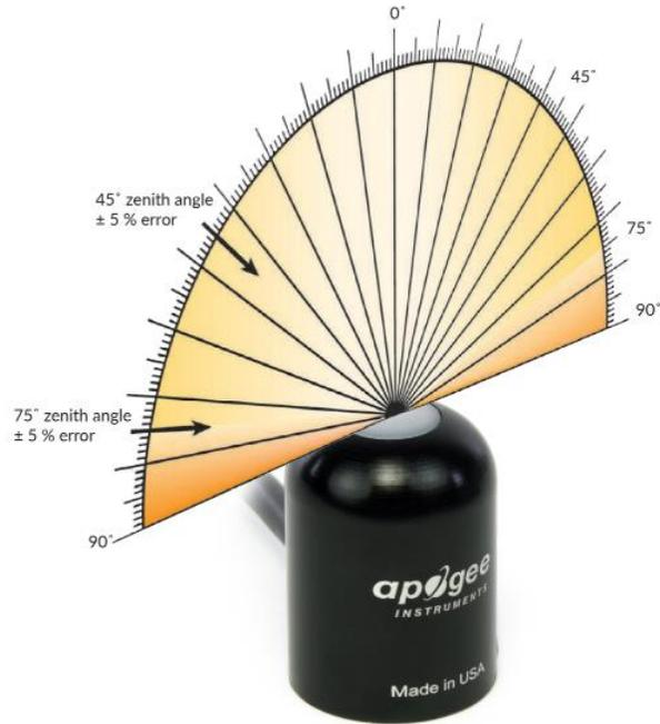
Directional, or cosine, response is defined as the measurement error at a specific angle of radiation incidence. Error for Apogee silicon-cell pyranometers is approximately ± 2 % and ± 5 % at solar zenith angles of 45° and 75°, respectively.
