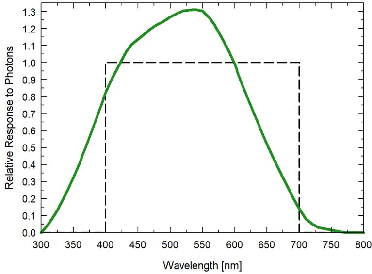
Mean spectral response of four SQ-100X series quantum sensors compared to PFD weighting function. Spectral response measurements were made at 10 nm increments across a wavelength range of 350 to 800 nm in a monochromator with an attached electric light source. Measured spectral data from each quantum sensor were normalized by the measured spectral response of the monochromator/electric light combination, which was measured with a spectroradiometer.
