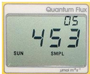
The LCD display consists of the total number of logged measurements in the upper right-hand corner, the real-time PPF value in the center, and the selected menu options along the bottom.
