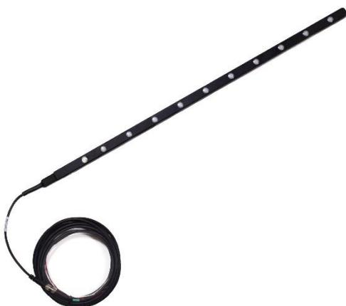
SQ-310X: Line quantum with 10 sensors and cable with pre-tinned pigtail leads
