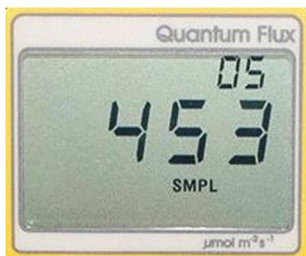
The LCD display consists of the total number of logged measurements in the upper right-hand corner, the real-time PFD value in the center, and the selected menu options along the bottom.
