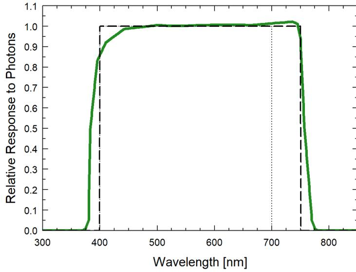
Mean spectral response measurements of four replicate Apogee MQ-600 series ePAR Sensors. Incremental spectral response measurements were made at 10 nm increments across a wavelength range of 370 to 800 nm in a monochromator with an attached electric light source. Measured spectral data from each quantum sensor were refined and normalized by comparing measured spectral response of the monochromator/electric light combination to measured spectral differences from a quantum sensor reference.
