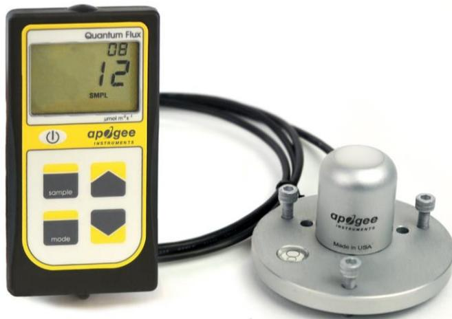
The AL-100 leveling plate is recommended for use with the MQ-610 (AL-100 leveling plate pictured). To facilitate mounting to a cross arm, the AL-120 mounting bracket is recommended.
