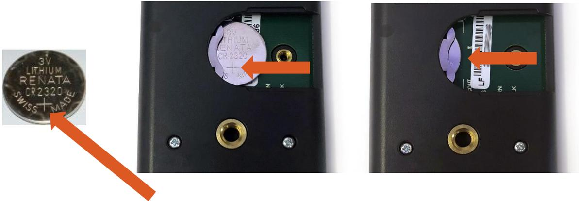
The positive side (designated by a "+" sign) should be facing out from the meter circuit board.
