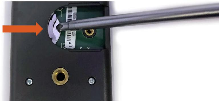
If the battery is difficult to move, turn the meter on its side so that the opening for the battery is facing downward and tap the meter downward against an open palm to dislodge the battery enough so that it can be removed with your thumb to slide the battery out of the battery holder.
