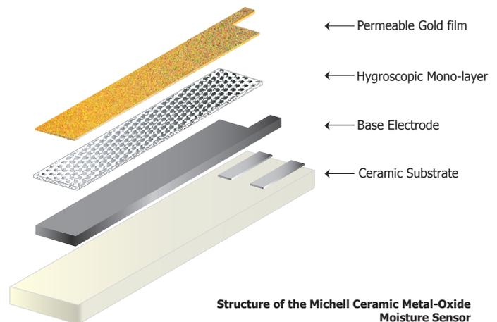
Structure of the Michell Ceramic Metal-Oxide Moisture Sensor
