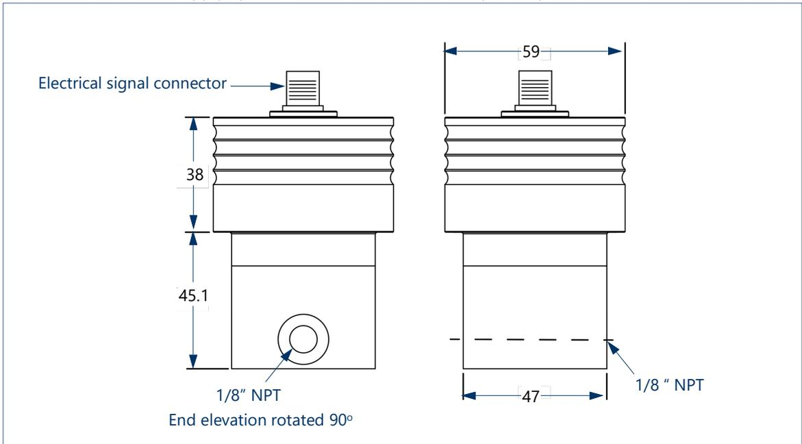
*Figure 5. Technical drawing of flow-through process connection*
