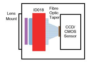
Alternative configuration for an Image Converter with integral CCD/CMOS camera for applications where direct viewing is not required.
