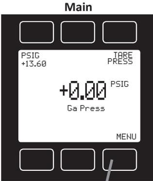
The **Main** display shows the pressure in the units specified at time of order. By hitting the **MENU** button at the bottom right of the screen you will enter the **Select Menu** display.
