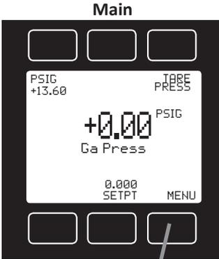
The **Main** display shows the pressure and setpoint in the units specified at the time of order.
