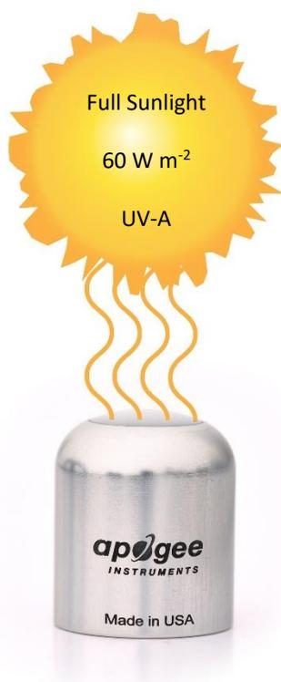
Example of UV-A measurement with an Apogee SU-202 sensor. Full sunlight yields UV-A radiation on a horizontal plane at the Earth's surface of approximately 60 W m<sup>-2</sup>. This yields an output signal of 1500 mV. The signal is converted to UV-A radiation by multiplying by the calibration factor of 0.04 W m<sup>-2</sup> per mV.
