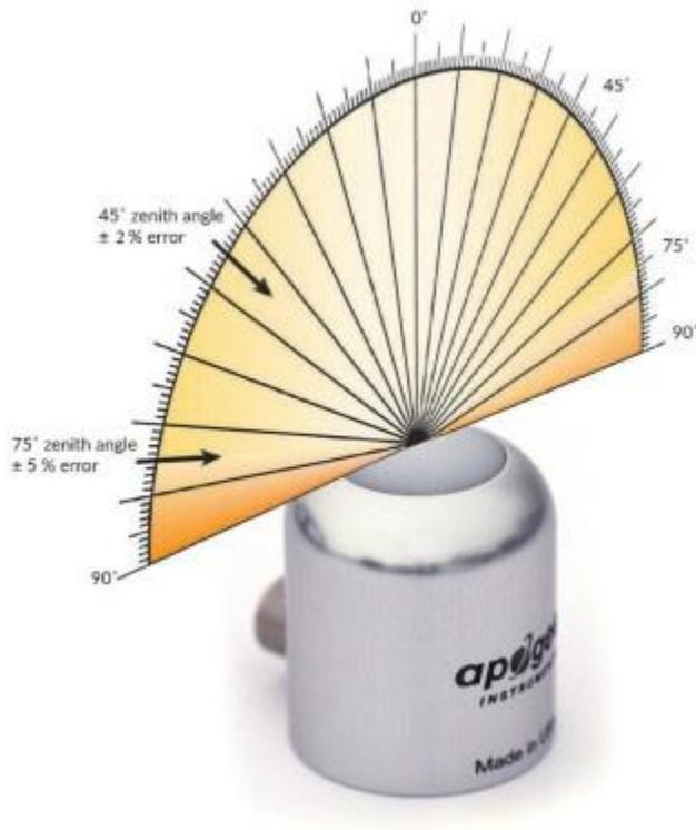
Directional, or cosine, response is defined as the measurement error at a specific angle of radiation incidence. Directional error for Apogee SU-200 series UV-A sensors is approximately ± 2 % and ± 5 % at solar zenith angles of 45° and 75°, respectively.
