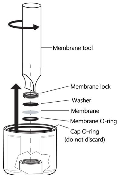
*Figure 8-1. Remove membrane and membrane O-ring*
