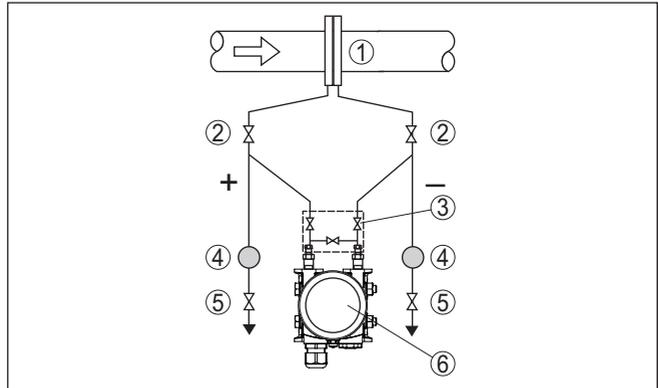
Fig. 19: Measurement setup, flow measurement in liquids
