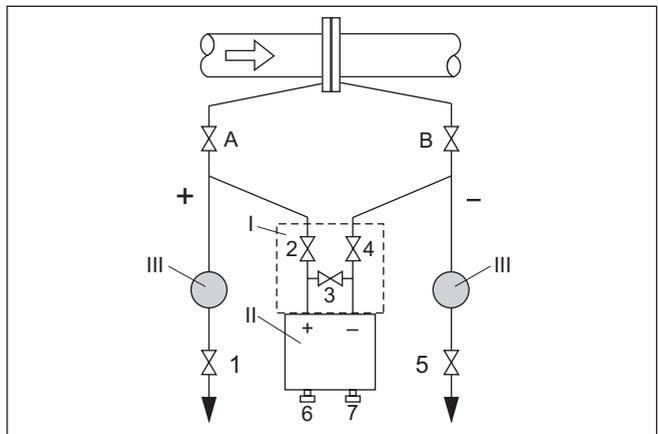
Fig. 38: Preferred measurement setup for liquids
