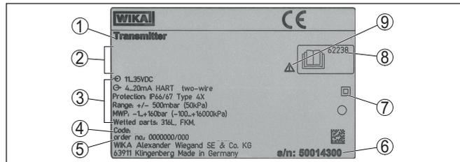
Fig. 1: Layout of the type label (example)
