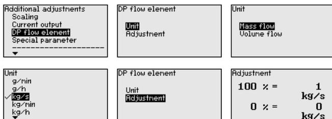
Furthermore the adjustment for the volume or mass flow rate at 0 % or 100 % is carried out.
