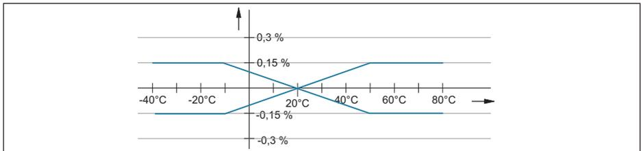
Fig. 42: Thermal change, current output
