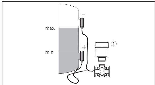
Fig. 15: Measurement setup, level measurement in closed vessel
