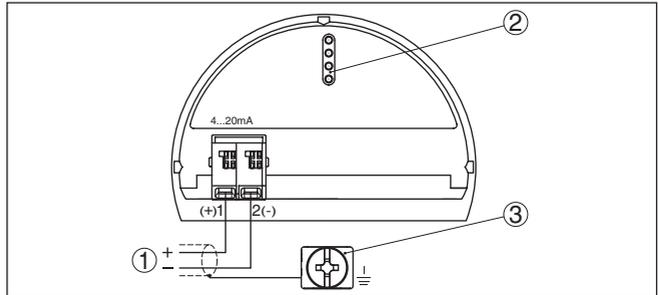
Fig. 27: Electronics and connection compartment - single chamber housing
