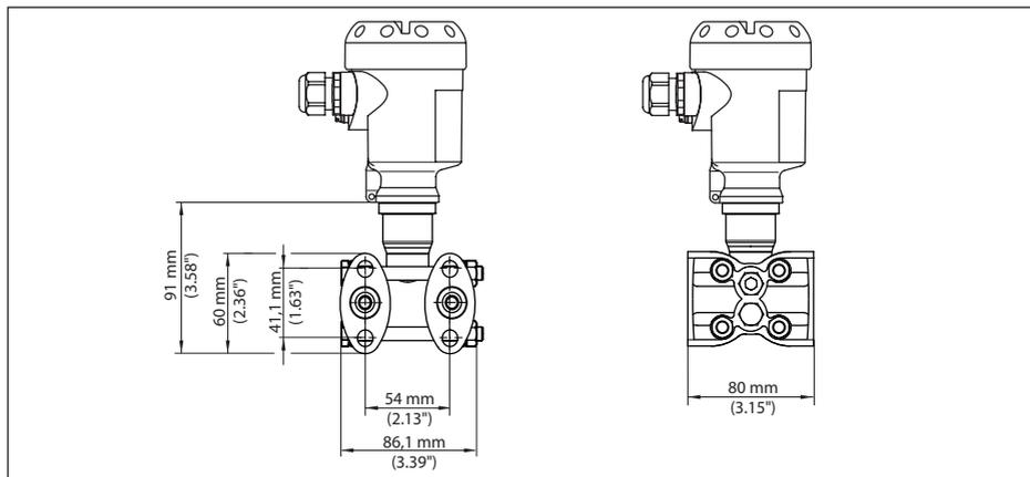
Fig. 46: DPT-20, ¼-18 NPT connection, with lateral ventilation
