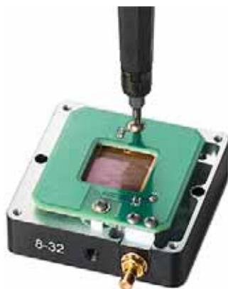
Figure 3-16. Attach Pass-Thru Circuit Board
