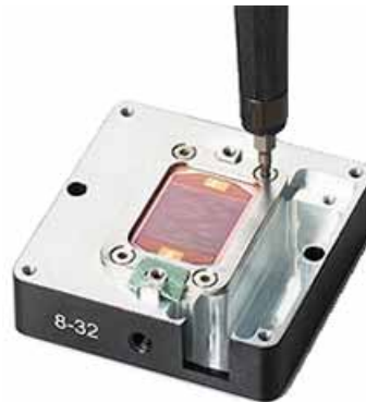
Figure 3-21. Remove Sensor Retainer (Frame)
