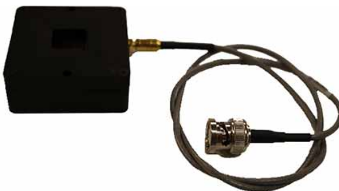
Figure 3-18. Attach SMB Cable
