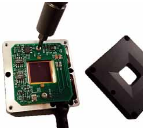
Figure 3-7. Unscrew the Circuit Board
