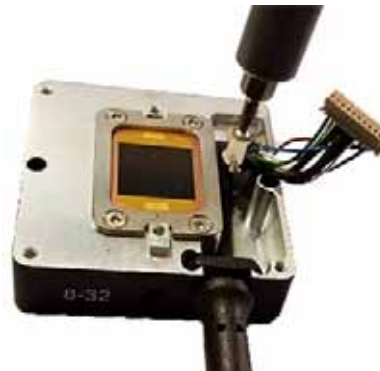
Figure 3-10. Unscrew the Ground Lug
