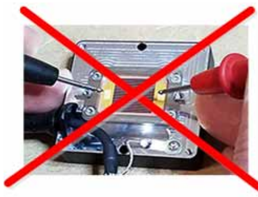
Figure 2-1. WARNING: Do NOT Probe the Sensor!
