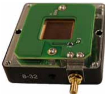
Figure 3-15. Align Pass-Thru Board in Sensor Housing
