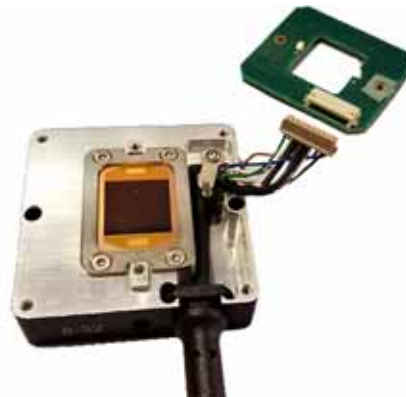
Figure 3-9. Disconnect the Circuit Board
