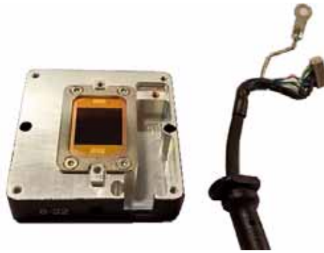
Figure 3-11. Remove Wiring Assembly from the Sensor
