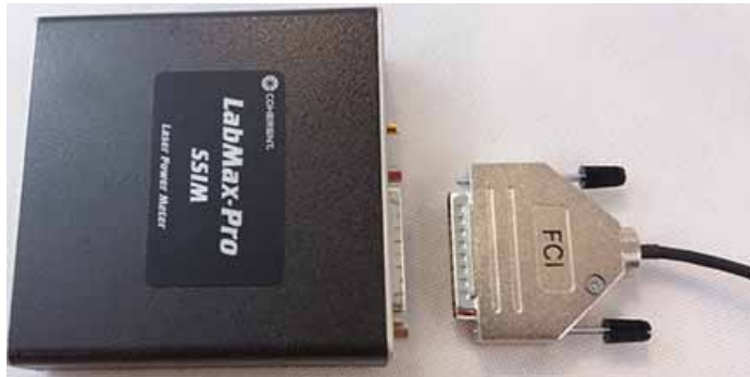
Figure 2-16. Connect the Sensor to the Meter
