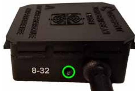
Figure 2-11. Sensor Post Attachment Option
